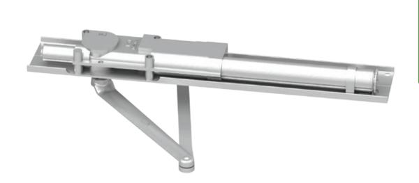
The concealed 5030 Series PACER® is a heavy duty closer designed to fit in a narrow, minimum 1-3/4" aluminum transom. The double lever arm provides superior door control and the choice of finishes and arm functions meet virtually all architectural requirements.
